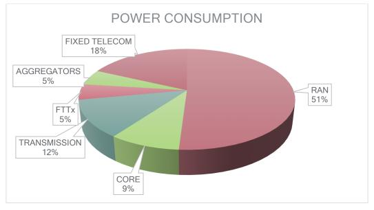
Figure (14) Power consumption of telecom access network
