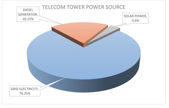
As per the findings, 76.25% of the towers were running on national grid, 20.15% on diesel generators, 3.6% on solar power as depicted in the figure (9) below.
