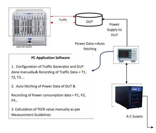
Figure (25) A typical test set up of Green Passport Lab
