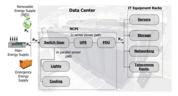
Figure (16) Power consumption at different layers of typical data centre
