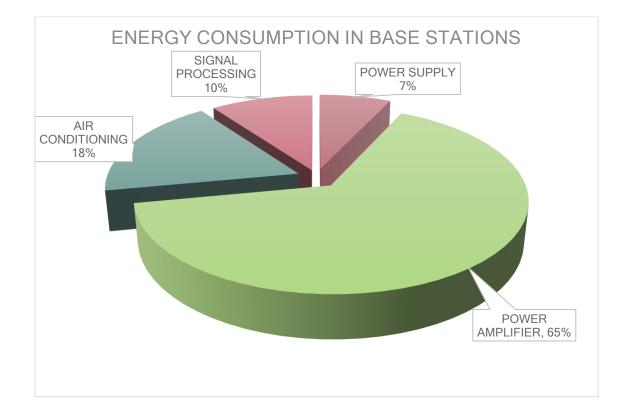
Figure (22) Energy consumption in base stations
