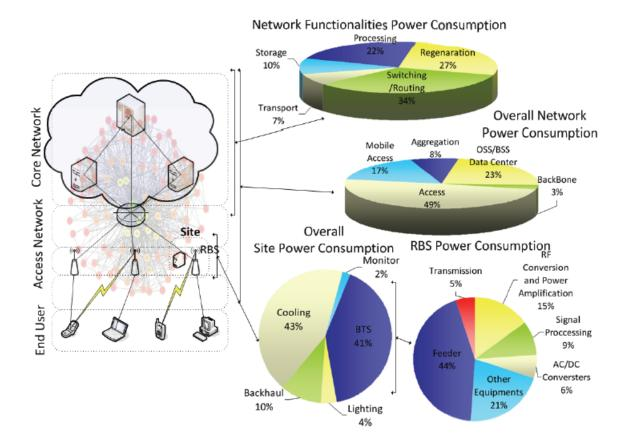
Figure (15) Power consumption in the different layers of a network
