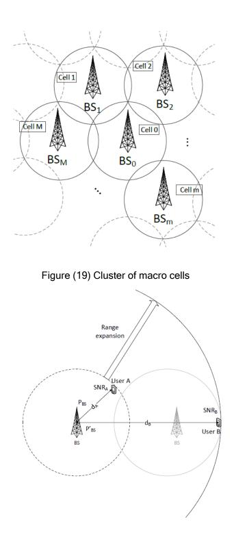
Figure (20) Increased coverage area of active cells
