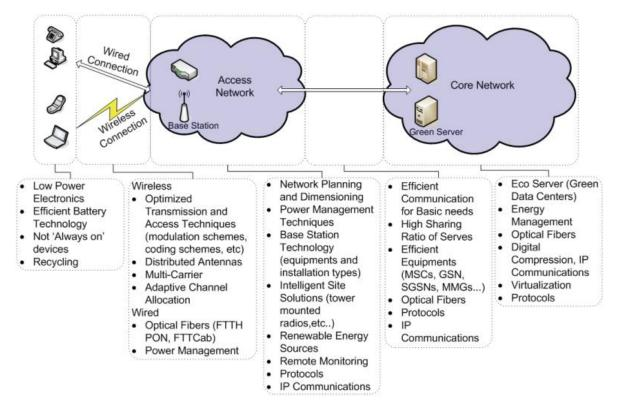
Figure (18) Energy efficient solutions of telecommunication networks
