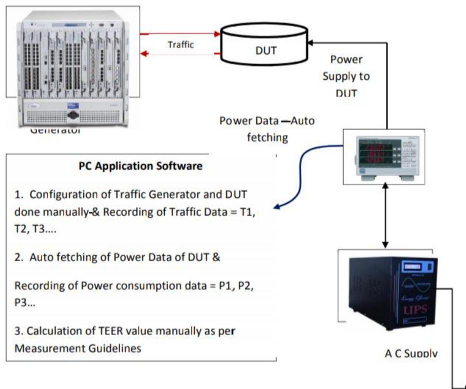
Figure (25) A typical test set up of Green Passport Lab
