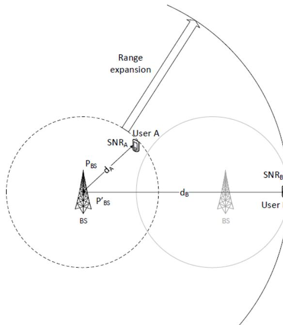
Figure (20) Increased coverage area of active cells
