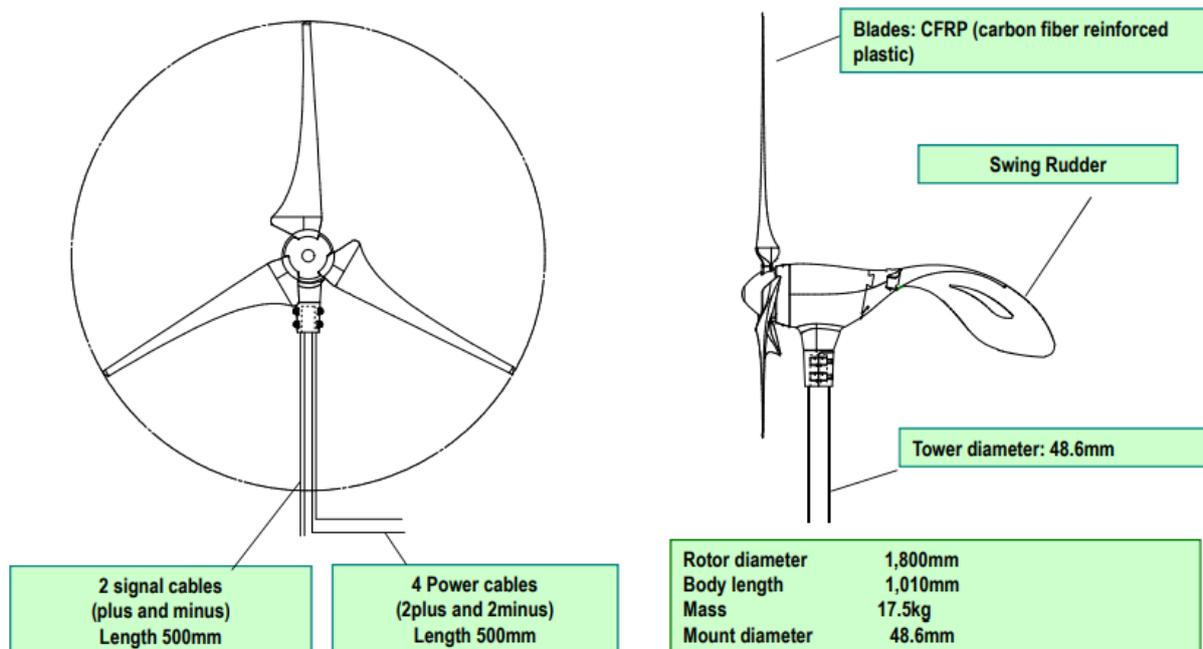
Figure (24) Wind energy turbine
