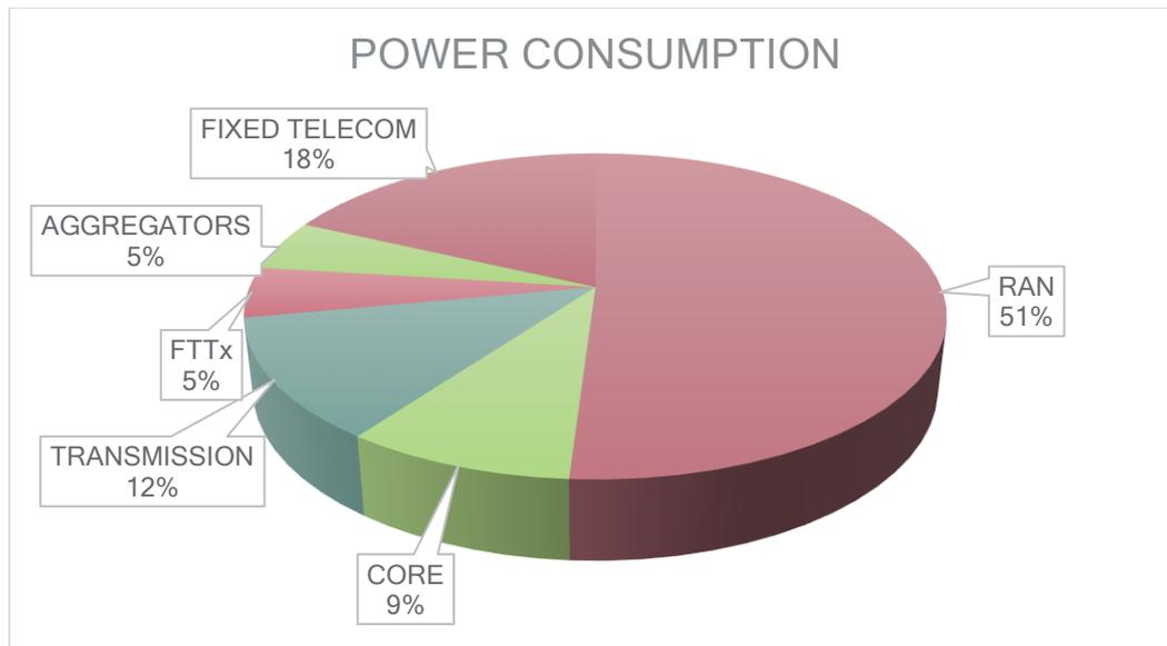
Figure (14) Power consumption of telecom access network
