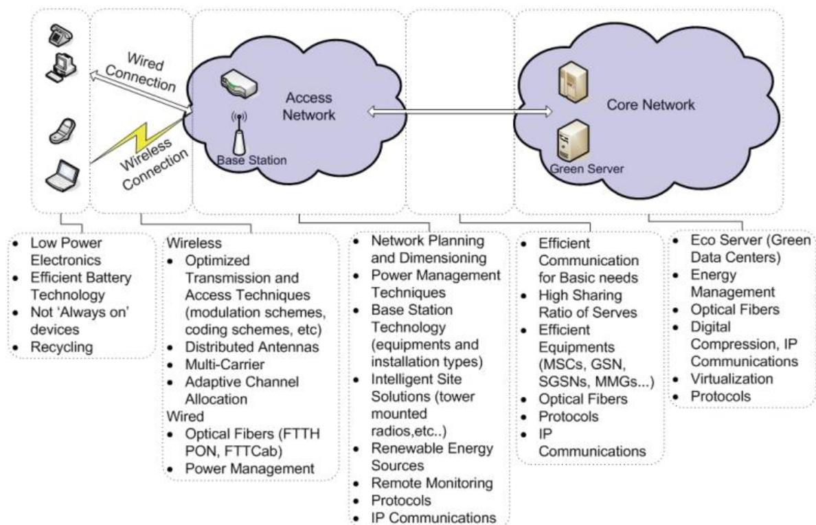
Figure (18) Energy efficient solutions of telecommunication networks
