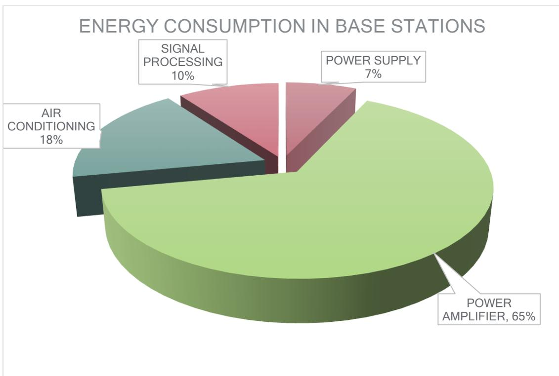
Figure (22) Energy consumption in base stations
