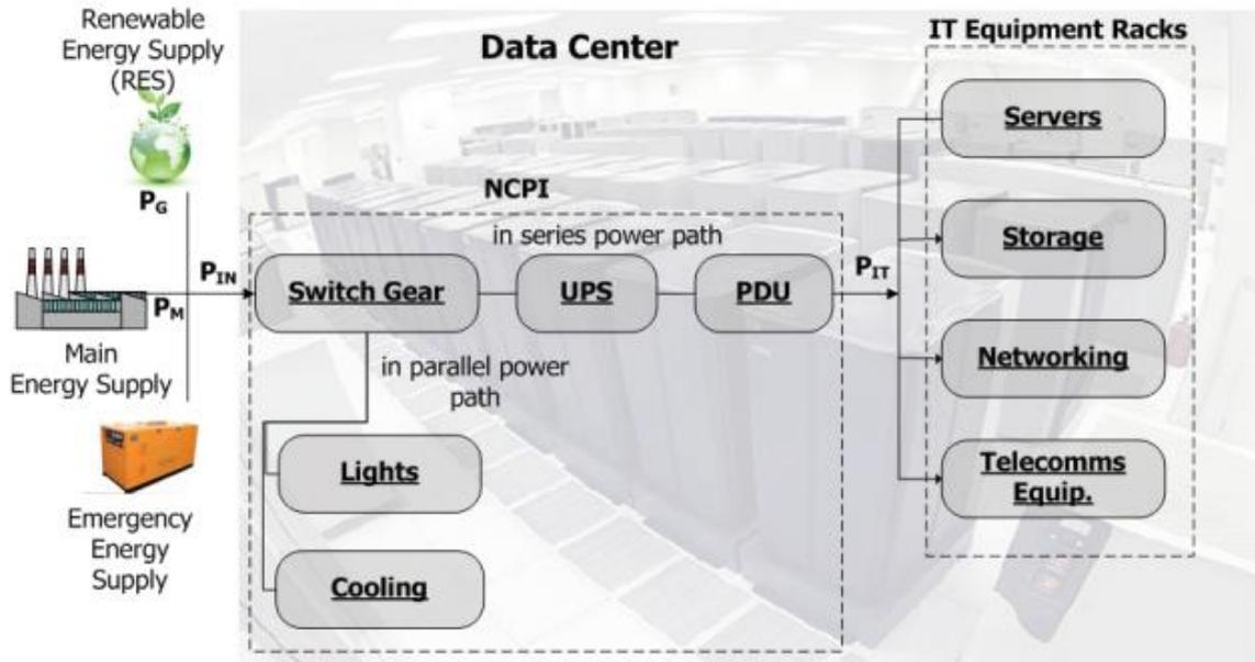
Figure (16) Power consumption at different layers of typical data centre
