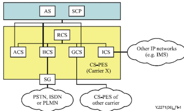
\* AS: Application Server, SCP: Service Control Point, SG: Signaling Gateway, PES: PSTN Emulation Service Component
