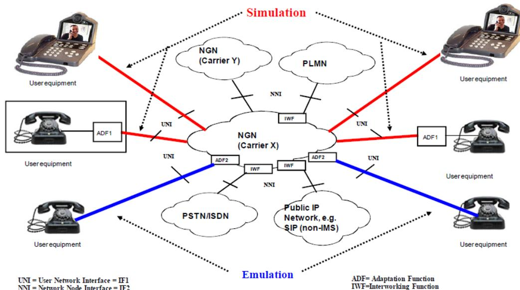
**Overall view of using NGN Emulation and Simulation**
